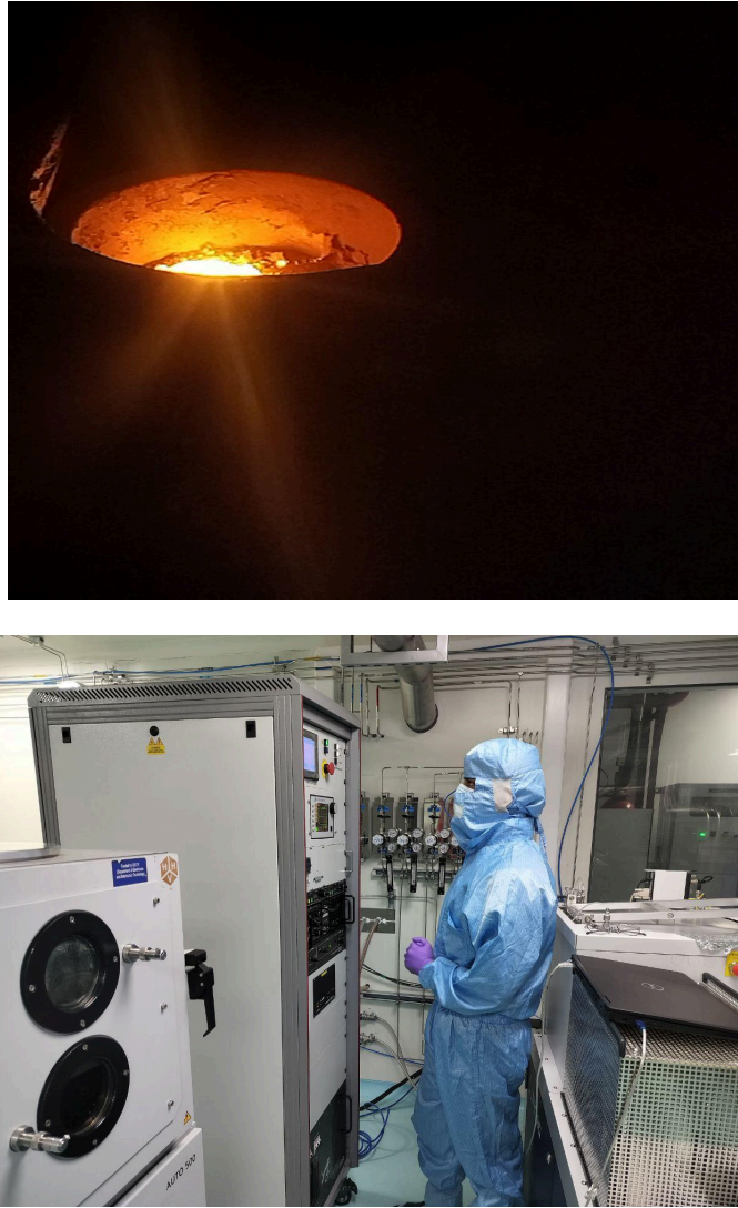
Fig 9 : Top-Gold being evaporated in the e-beam apparatus; Bottom-Operating the E-beam evaporator
