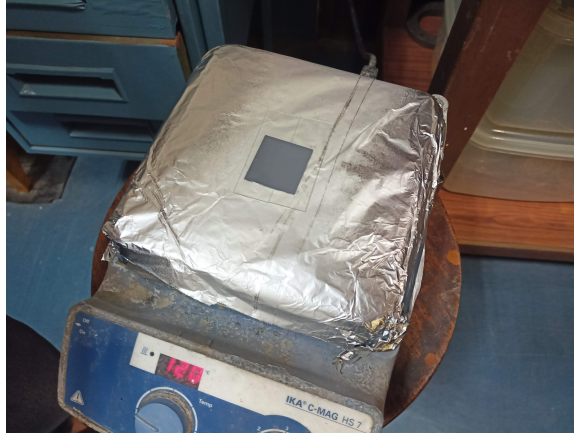
Figure 2.3: Preheat treatment of a textured wafer
