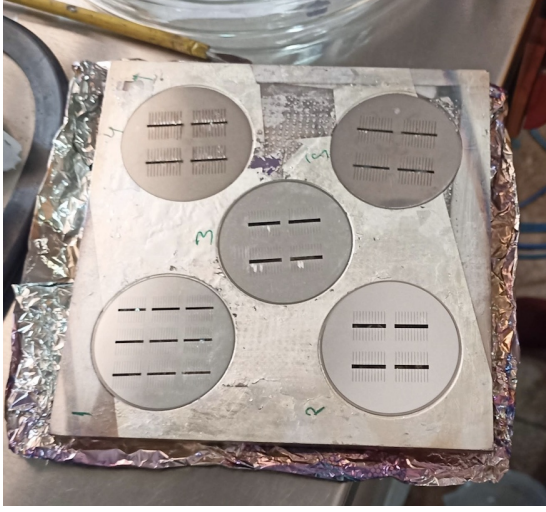
Figure 2.6: Masks for thermal deposition
