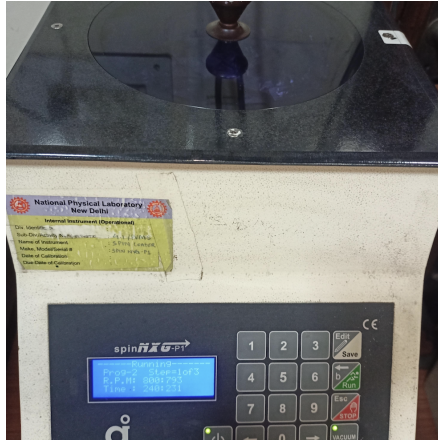
Figure 2.4: Wafer being spin-coated
